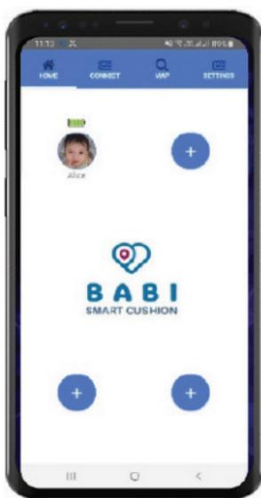
The battery charge indicator will change color as battery charge lowers. When the battery is critically low this icon will become red. Whenever the sounder sounds 4 times, it is an indication that the battery needs replacing; also a notification will be showed if phone screen is off. To complete the App setup, press the Settings icon on top right corner here it is possible to enable the vibration, the intermittent flashing light and to select a preferred alarm tone.
